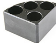
Black quarter pie, 4 holes, 40mL reaction vessel, \varnothing 28\text{mm} , 43mm depth
